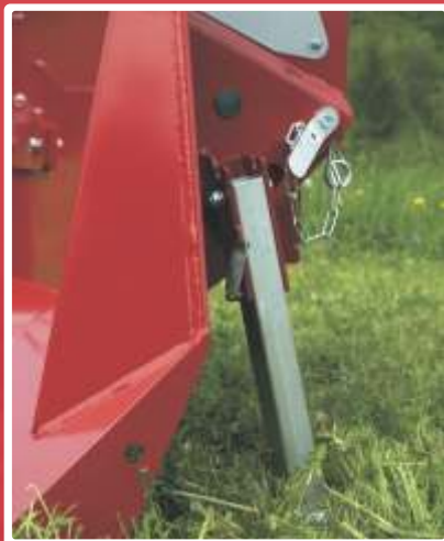
Two folding support legs for stability when disengaged from the tractor
