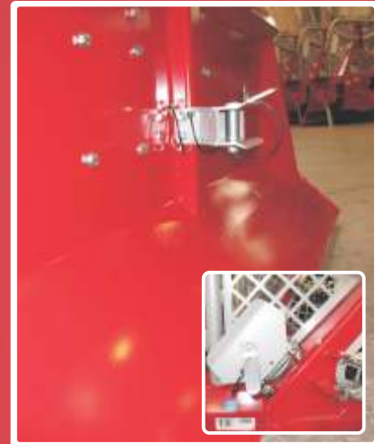
Coupling - mounted in series removable via locking pins
