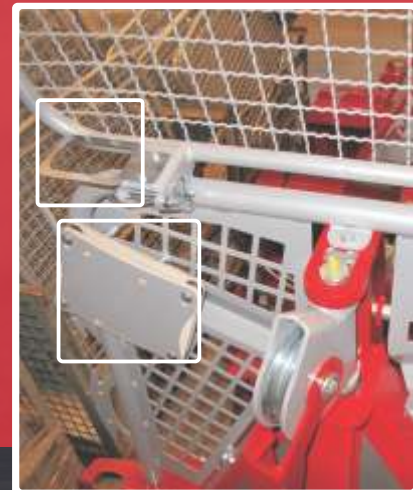
Folding wireguard Holder for motor saw Holder for tail hook
