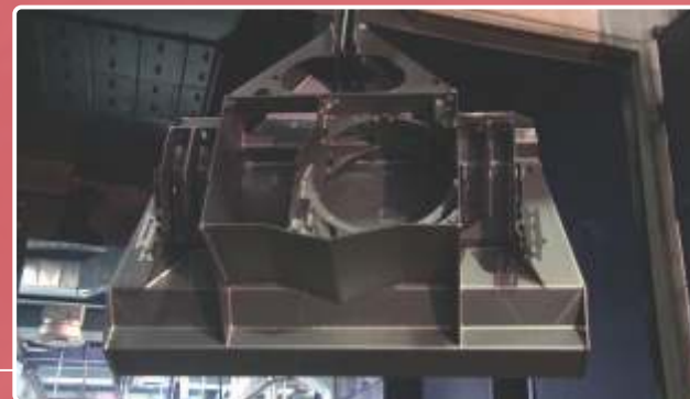
Before painting, we clean and debur them in a sand chamber, thus achieving an excellent surface structure for the dry spray system of lacquering.
