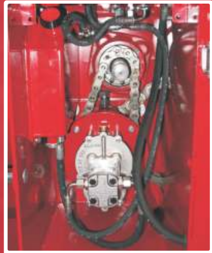
Hydraulic pump driven by a multiplying gearbox
