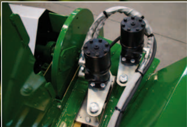
2 powerful hydraulic motors secures a strong and aggressive in-feed.
