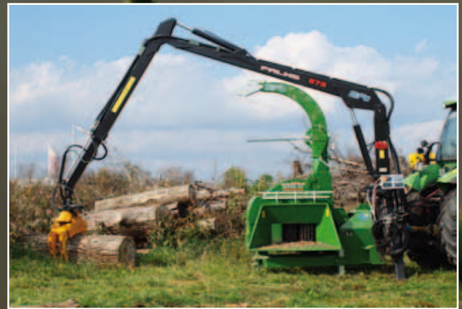
NHS 300icv is a 90° machine. Crane feded 90° in the direction of driving.
