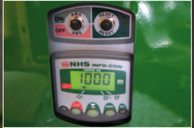
NHS InfoCon is a combined Antistress, Hour Meter and service interval counter. Available for all models.
