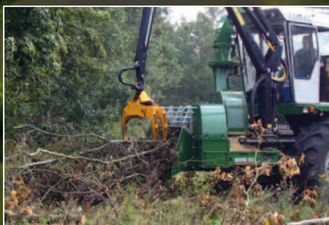
The NHS 450f in-feed handles whole trees, even trees with big crowns.
