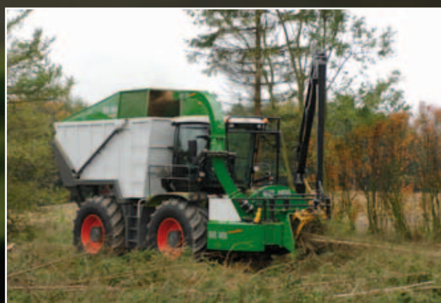
Claas Xerion with standard NHS 450f – 6m crane – NHS grip – 16 m 3 collector box.
