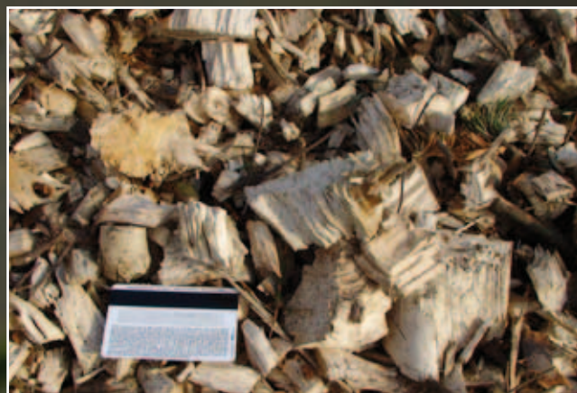
NHS 450f produces 35 mm chips. The chips are documented for use in CHP and heating plants.
