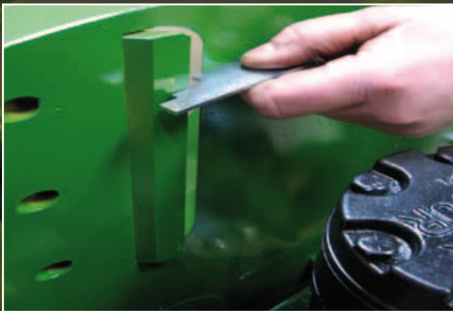
Knives on most NHS standard machines can be adjusted stepless
