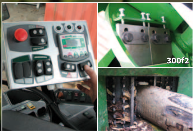
Forestline control box. Split knives for optimal operating cost. Aggressive vertical in-feed rollers.
